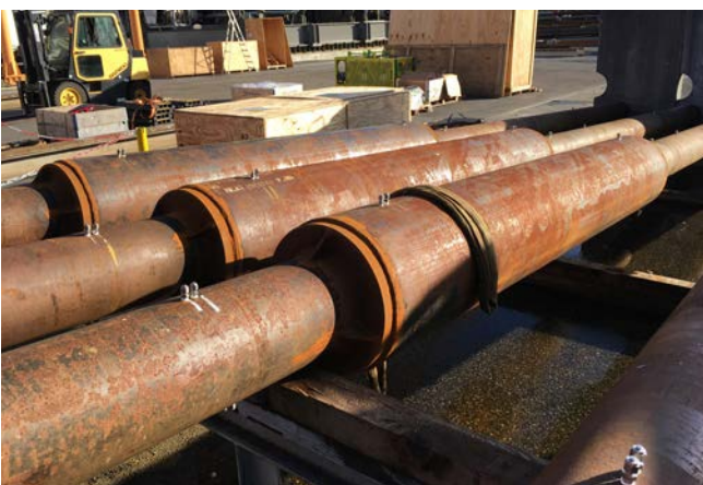
The four test assemblies constructed with 7" tubing inside 9 5/8" casing and 16" washout section.
