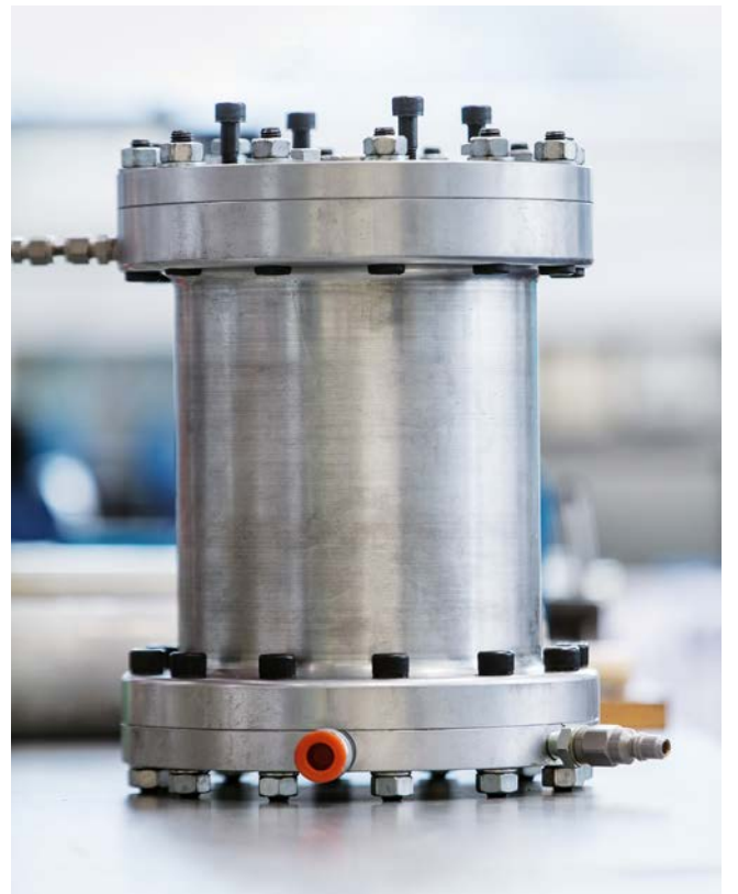
Laboratory set-up for experimental tests of cement sheath integrity.
