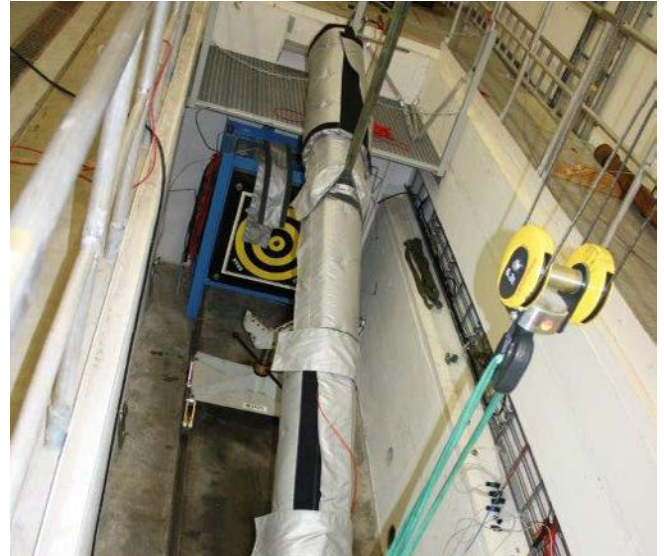
Noise logging experiment using sound proofed reference cells installed in the Ullrigg HETE test pit.
