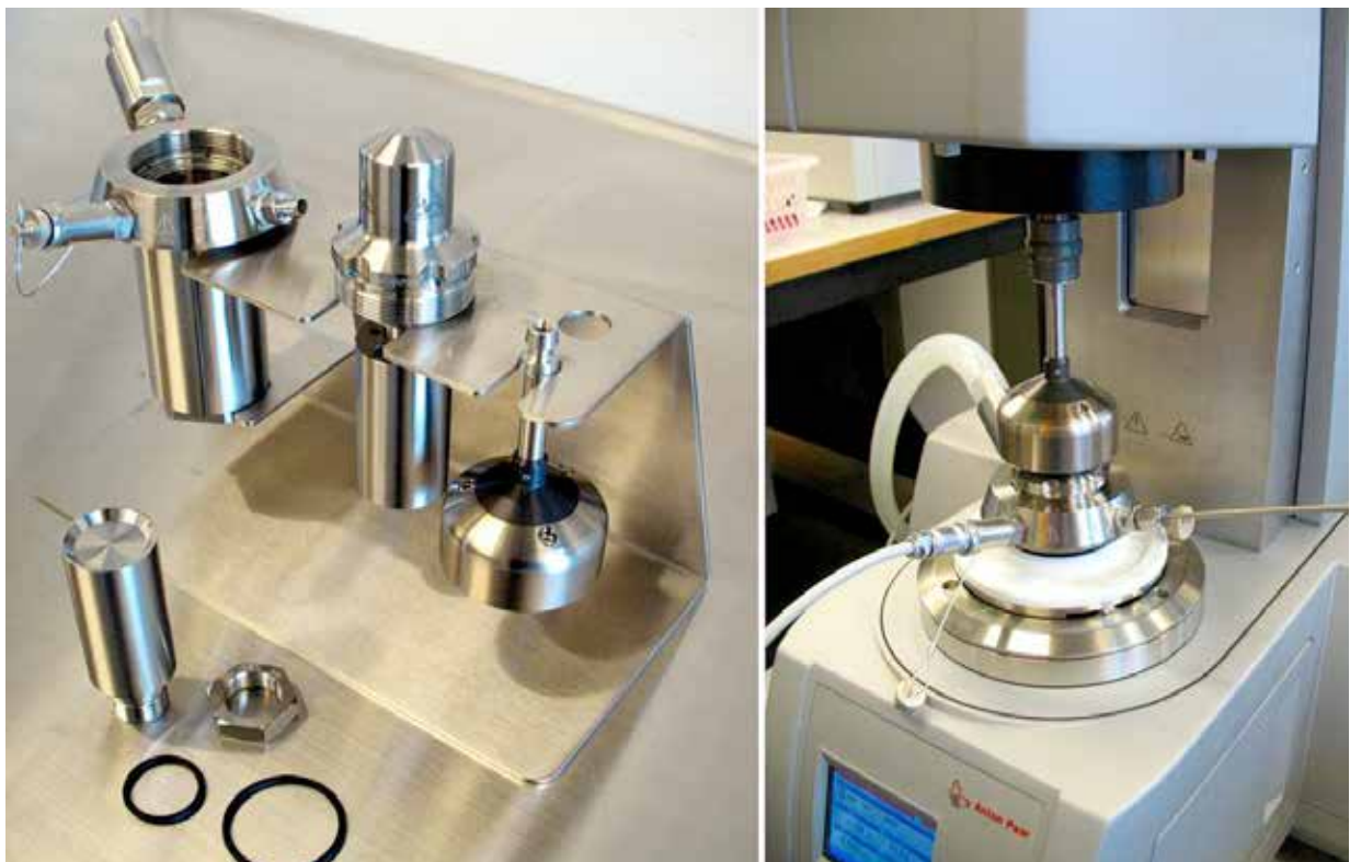
Figure 1: Left: The components of the double-gap cylinder pressure cell used for measurements of viscosity and shear stress at pressures up to 200 bar. Right: The pressure cell is shown mounted in the MCR 302 rheometer.
