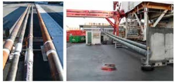
Figure 3: Full scale tests to determine if a good seal can be obtained after P&A when tubing is left in hole.
