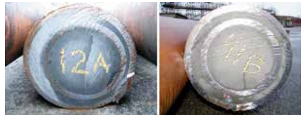
Figure 4: Cut strings with tubing cemented inside casing with and without control lines.
