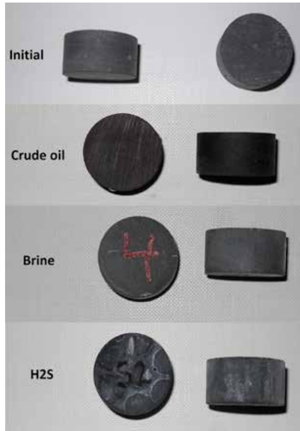
Figure 1: Cement samples after exposure to downhole environments at elevated temperature and pressure.
