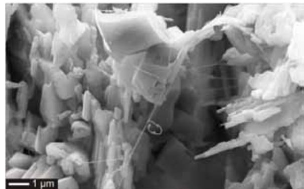
Figure 2. Half of the core freeze-dried. Inlet side. Well-preserved structures, with – partly network forming – polymer chains intact.
