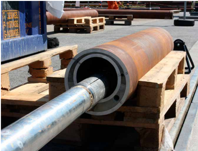
Logging survey inside a cement reference cell with drilled defects.
