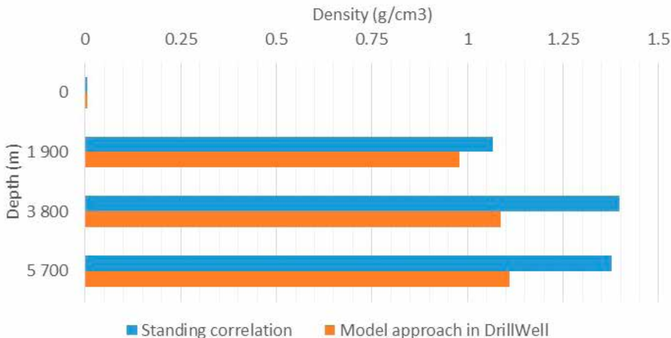
Density vs. depth, OBM with 8.82% (weight) methane
