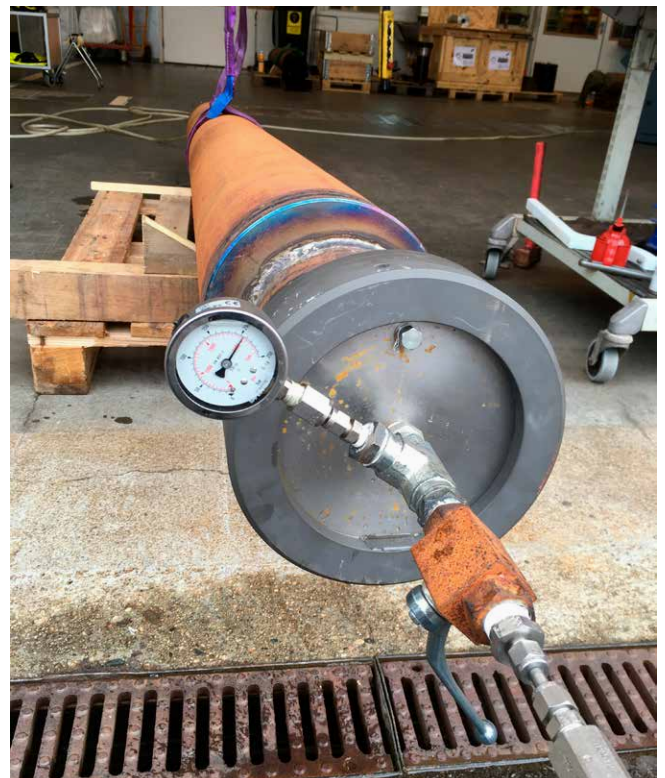
Pressure testing a barrier logging reference cell
